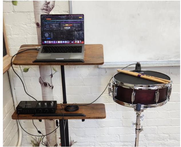
Figure 2: A Sensory Percussion setup, featuring a snare drum, the EVANS Portal, and a laptop running the Sensory Percussion 2 software application
