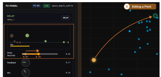
Figure 6: Variant editing selected point in the map (right) is opened in the FX panel (left), where users directly manipulate effect parameters (e.g., delay time, feedback, mix) to iteratively refine the sound and save an updated variant.
