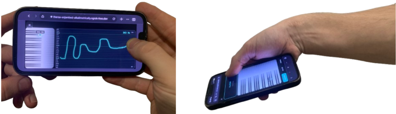
Figure 1: The two mappings of VoixTenu, Draw mode (left) and Gyro mode (right). In Draw mode, the output frequency is modulated by the vertical position of the user’s finger on the phone’s touchscreen. In Gyro mode, the pitch-axis tilt of the phone controls the frequency while the roll-axis tilt controls the volume of the output sound.
