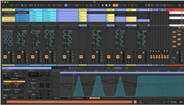
Figure 7: Ableton Live Session View. Grouped tracks synchronize audio clips with MIDI CC-based lighting automation, managing scene progression in Space A.
