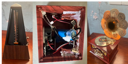
Figure 9: Interactive props for Space A and B. Left/Right: Modified vintage metronome and music box. Center: Internal view showing the embedded ESP32, MPU-6050, and transducer for on-board audio.
