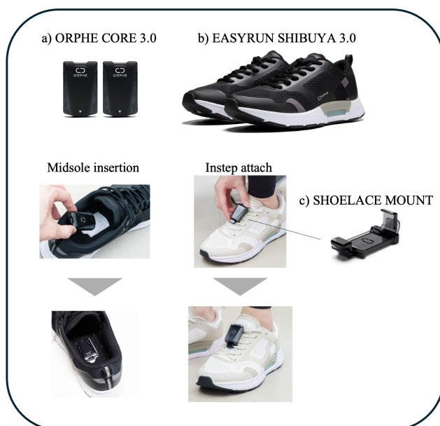
Figure 1 : Hardware configuration of the smart footwear platform. (a) ORPHE CORE 3.0: Small 6-axis motion sensor device. (b) EASYRUN SHIBUYA 3.0: Dedicated shoes capable of embedding the device inside the midsole. (c) SHOELACE MOUNT: Attachment capable of fixing the device to existing shoelaces.
