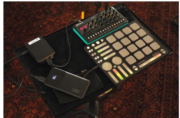
Figure 7: An intelligent setup of the Roland S-1 and Keith McMillen QuNeo interfaces with a Raspberry Pi 5 as used in festival performances in January 2026
