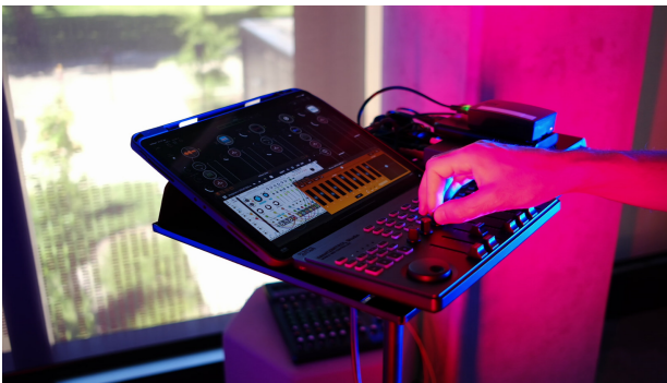
Figure 6: Software synthesisers used in an intelligent instrument setup. Digital audio workstation (DAW) software ran on the iPad which is connected via MIDI to the generative AI system on a Raspberry Pi 4. A performer can interact with the instrument using the iPad touchscreen or a hardware controller interface.
