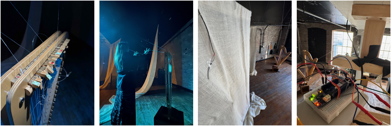
Figure 2: Augmented Harp-E structure: (a) the lever micro-tonal system on Harp-E and fishing lines on the lever for instrument augmentation, (b) harpist interacting with the augmented part of Harp-E with the same performance gesture as harps, (c) flex sensor attachment, (d) system dataflow transferring with Arduino.
