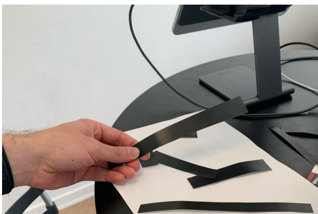
Figure 2: Contrast-based synthesizer: dark paper shapes placed on white background modulate oscillator waveform via brightness scanning.
