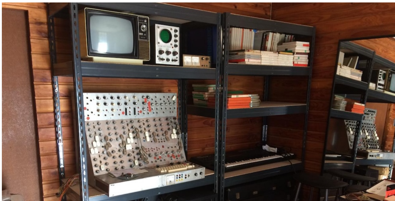
Figure 1: Frontal view of the Comdasuar. The instrument integrates a frontal control panel populated with numerous rotary knobs, switches, and patch points for real-time manipulation of synthesis parameters, alongside a keyboard interface for symbolic input. A black and white TV was used as a visual display for the device.
