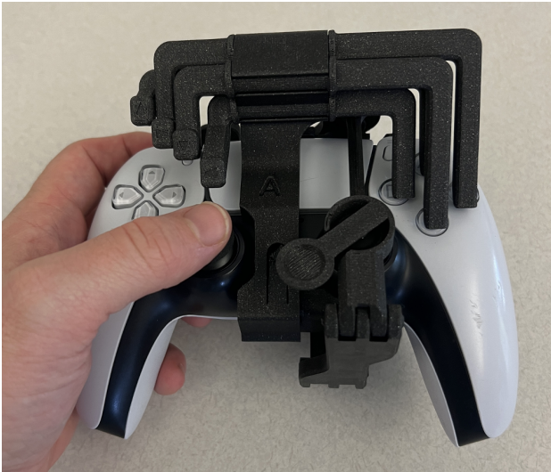
Figure 1: A DualSense controller augmentation for one-handed operation, design files freely available on Printables.
