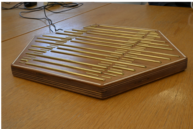
Figure 3: Design of Reharp, where sound triggered by touching the metal rods
