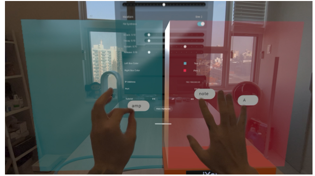
Figure 3: Screenshot of the iXeRemin interface showing the semi-transparent boundary box and real-time fingertip labels for amplitude, note-on/off state, pitch or chord name.
