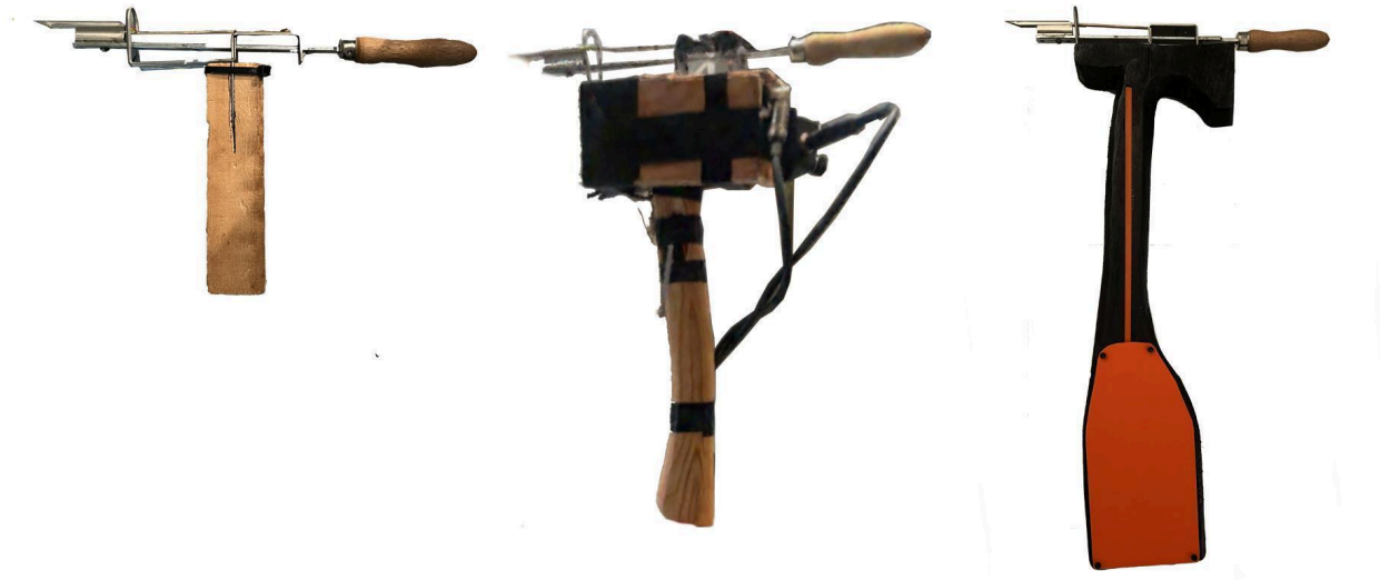
Figure 1: Pictured from left to right, V1 carpet tufting tool, V2 carpet maker's hammer, V3 Carpet Maker's Hafted Tool (CMHT)
