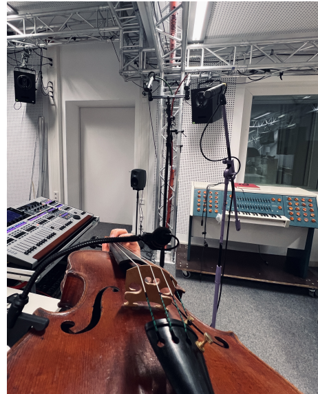
(b) Violist's point of view during recording. The DPA clip-on microphone attached to the viola records high-quality audio, whereas the reference microphone is on the microphone stand in front of the musician. Also visible is a stereo-pair of microphones. We chose to model mono audio signals and therefore we did not use the audio from this stereo pair in the final dataset.
