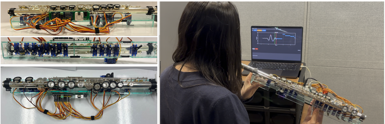
Figure 1: Overview of the ensemble performance setup using the developed semi-automated robotic flute and the gesture-cue-based control system with MIDI accompaniment.
