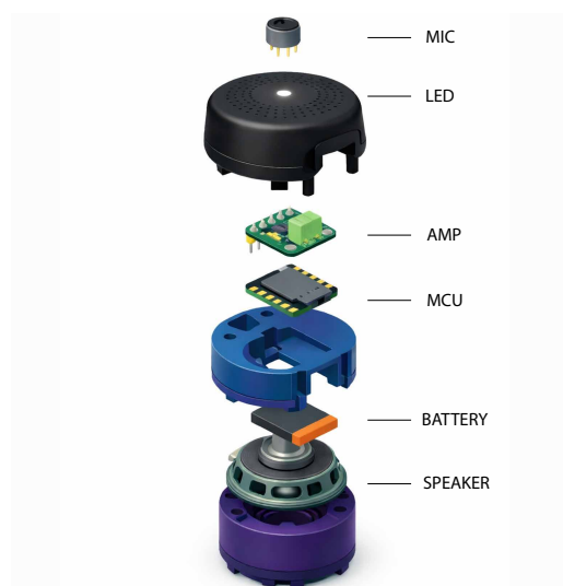
Figure 6: Exploded Sound Swarm node showing the MEMS microphone, status LED, ESP32-S3 MCU, audio amplifier/DAC, LiPo battery, speaker, and enclosure.
