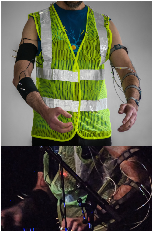
Figure 3: [Above] The vest interface. Interior breast pockets left and right hold pre-amp/transceiver module and the TENS device. Electrodes for TENS (left) and EMG (right) are held by elastic straps. [Below] Video still of the vest in use. (from video: https://www.dorftv.at/video/45716 ).
