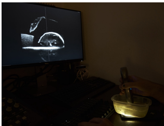
Figure 2: Scanning of a gelatin phantom with a linear probe. The onscreen vertical line is the current position sampled by the IFFT. The suspended forms here include tofu, grape and orange peel.
