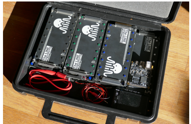
Figure 6: Carrying case ( 27 \times 37 cm) capable of accommodating up to eight modules (64 loudspeaker), together with the FPGA unit and the power supply.
