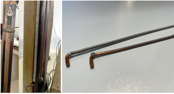
Figure 9: Original wirewound sensors at XK instruments.
