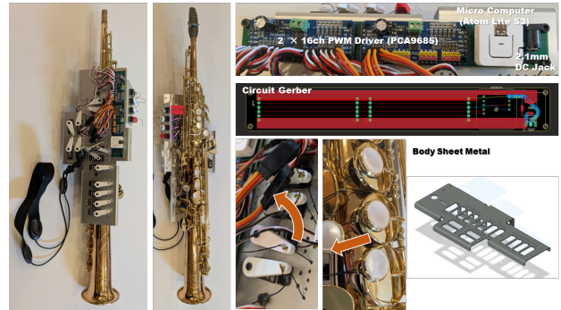
Figure 2: Robo-soprano saxophone with an attached robotic key-actuation module. Nineteen servo motors and a compact control circuit are integrated into a high-rigidity anodized aluminum body, enabling reliable key actuation
