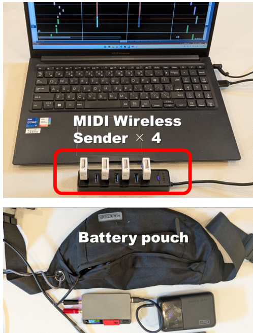
Figure 5: Wireless communication and portable power system for the robo-sax quartet. Top: Four wireless transmitters connected to a PC via a USB hub, each corresponding to one robo-saxophone (soprano, alto, tenor, and baritone). Bottom: Wearable battery pouch integrating a mobile power bank and DC regulator, enabling stable power supply without restricting performer movement.
