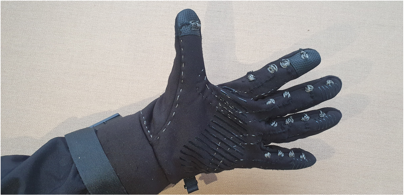
Figure 1: Layika, a wearable glove-based interface that maps traditional hand-based Taal counting gestures to Tabla accompaniment during solo vocal practice.
