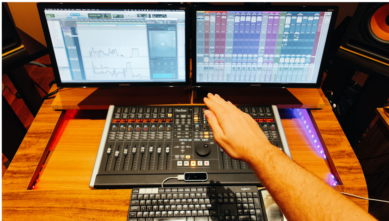
Figure 1: Leap Motion Controller being used to control spatialization in Dolby Atmos format.
