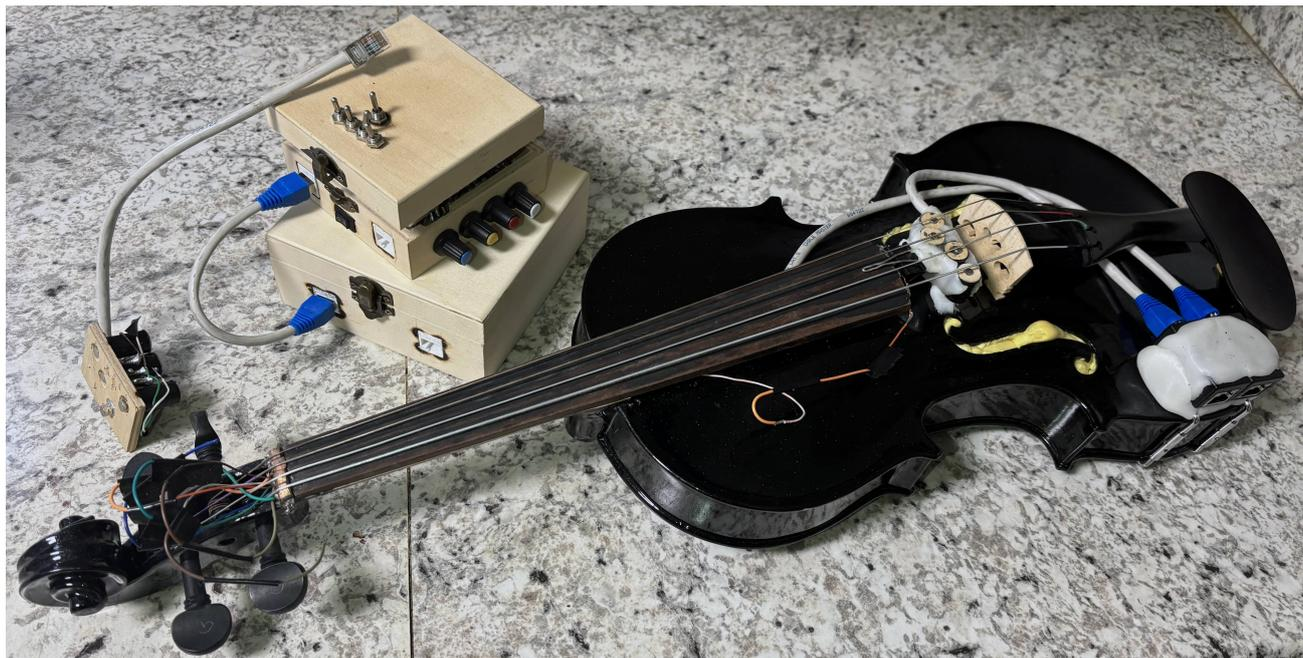
Figure 1: EV 1 with two processing boxes and its initial pickup.
