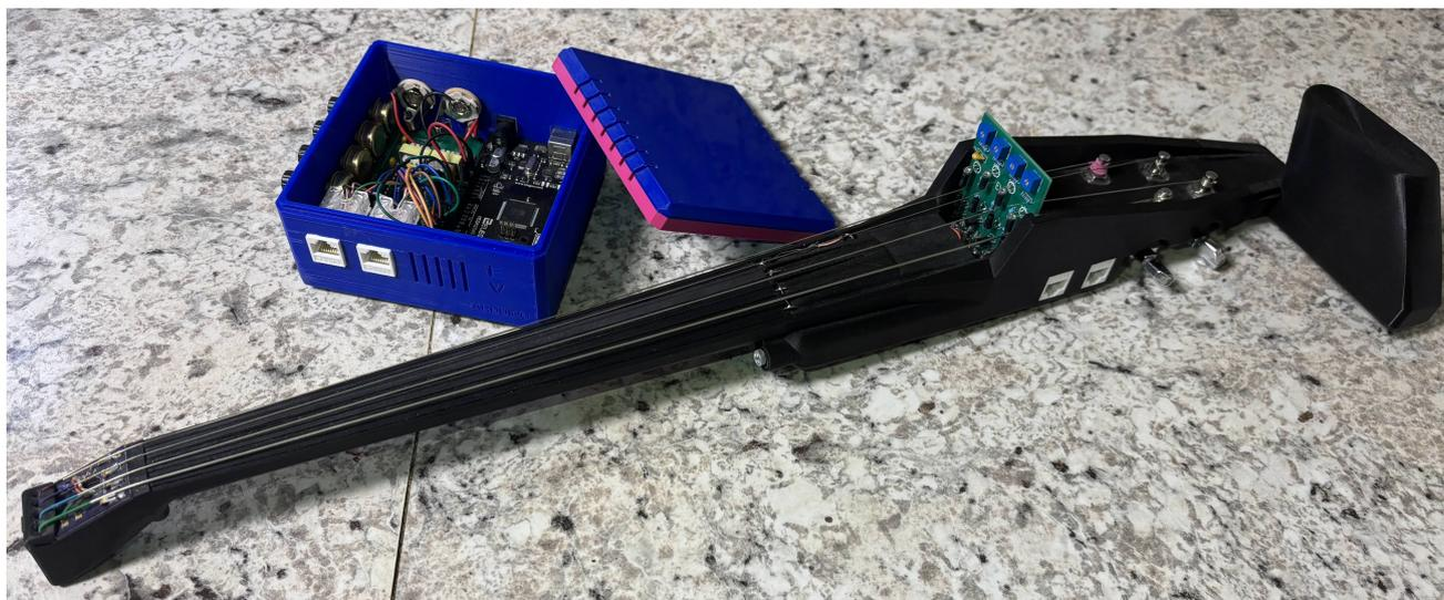
Figure 2: EV 2 with a processing box housing an Arduino and preamplifier.
