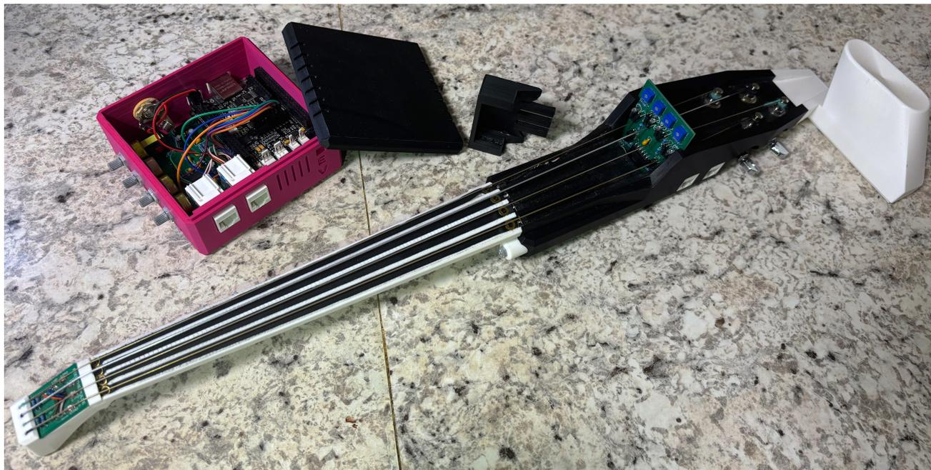
Figure 3: EV 2.5 with a processing box housing a Bela and preamplifier. Also shown is the hood for the IR pickup
