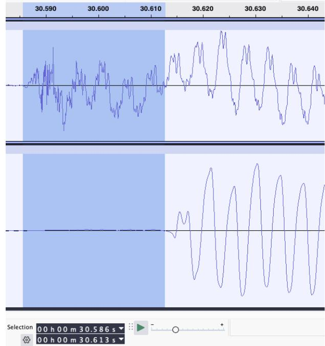
**Figure 6: EV 2.5 Latency Measurement of 27 ms. Top track: EV string recorded via a microphone directly. Bottom track: the EV string via the IR pickup and passed unchanged through the EV system and output through a speaker.**
