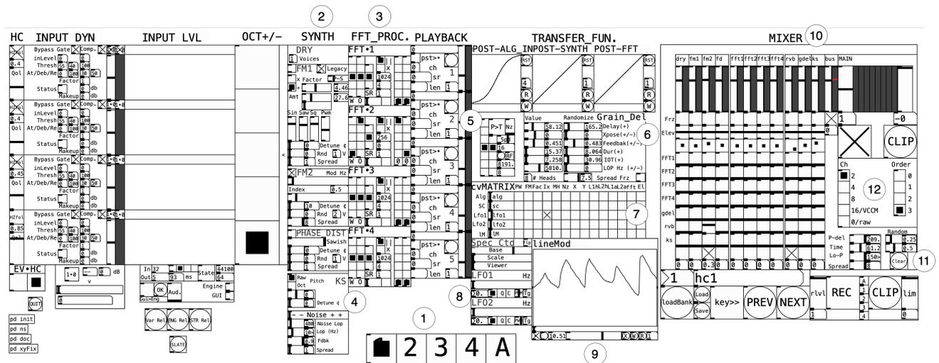
Figure 5: EV’s GUI. 1) Current string displayed. 2) The three synthesizers. 3) Four FFT convolution engines, with settings for sample rate, overlap, window size, input swap, and source selection. 4) Karplus-Strong effect. 5) Buffer freeze, with settings for overlap, window size, playback rate, and refresh. 6) Granular delay. 7) CV matrix. 8) LFOs. 9) Envelope generator. 10) Mixer. 11) Reverb. 12) Ambisonics options.
