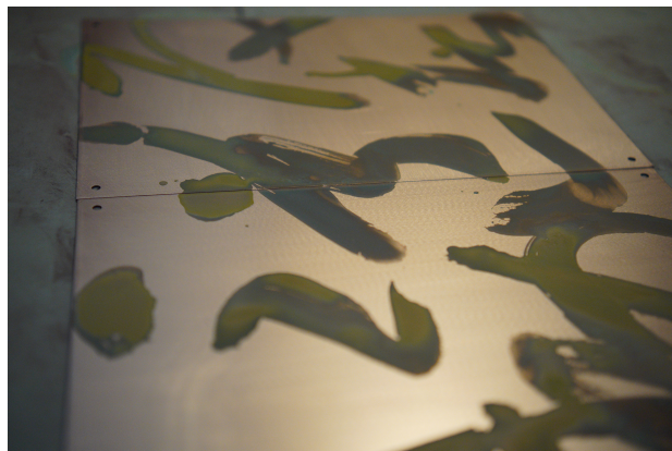
Figure 3: Growth of patina, 2 minutes after applying the acid.
