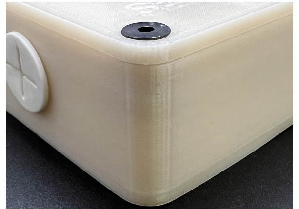
Figure 7: 3D-Printed Enclosure with Algae-Based Filament.
