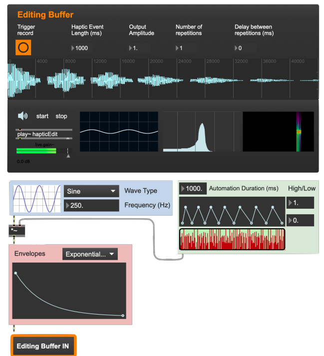
Figure 2: Tactile tremolo created with the haptic toolkit.
