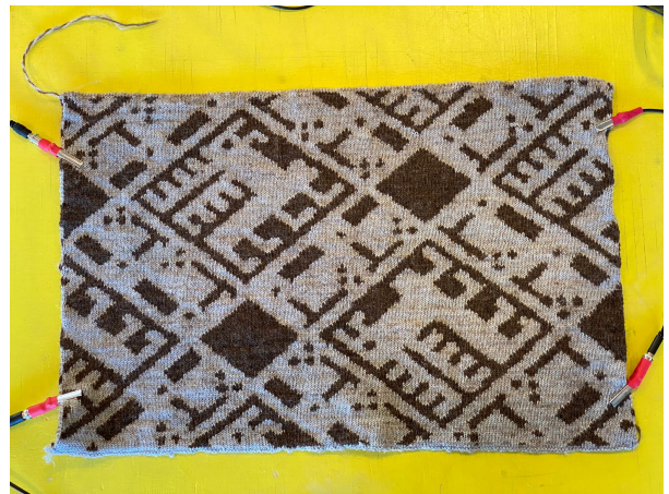
Figure 2: The ‘Knitted Mat’ interface with the positive-negative Jacquard pattern, the lighter one including the piezoresistive yarn.
