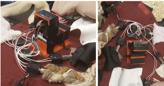
Figure 3: 3D printed cases storing the Bela and the 3.5mm jack connections inside the centerpiece of the artifact. The cases are stitched to the centerpiece, securing the Bela and the jack connections from abrupt movements.
