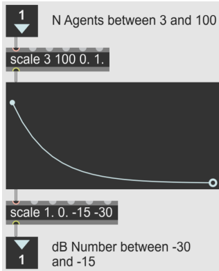
Figure 6: Gain attenuator for the “sound swarming” output. It shows how the signal gain in decibels (dB) changes based on the number of agents, using a drawable decaying curve.
