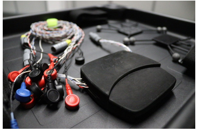
Figure 1: Data acquisition platform: 8-channels sEMG wearable sensor board. Two sides, four channels for each side.
