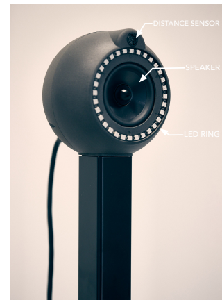
Figure 4: Closeup image of the individual singer, showing the location of the speaker, ultrasonic distance sensor, and LED light ring.
