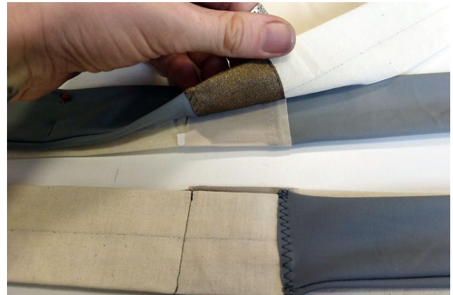
Figure 4: Layers in the shearing sensor, showing the corresponding layers of conductive fabric in the centre in gold, lower one with an added a layer of pink powermesh to isolate the two conductive panels.
