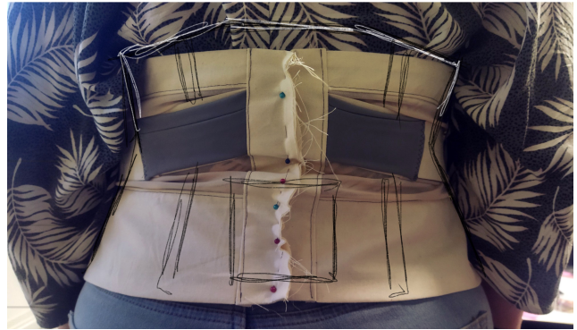
Figure 6: Annotated toile-in-progress: Implementing the abdominal (top) and back (bottom) shearing sensors around areas of expansion in Reed’s body into the unfitted toile.
