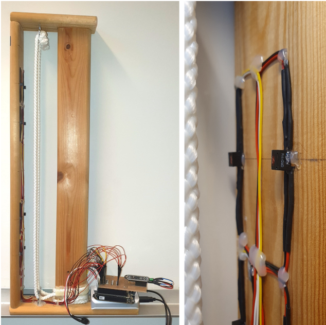
Figure 4: The CordChord. Left: The side profile showing the rectangular wooden frame with 2 ‘cords’ of polyester rope fixed between the short sides. Right: A closer view of distance sensors mounted on the neck facing towards the cords.
