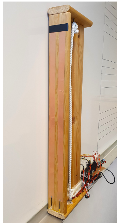
Figure 7: The copper capacitive strips on the back of the neck, facing towards the performer.
