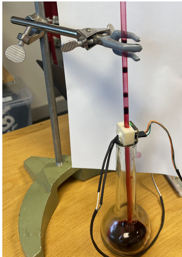
Figure 4: Synthetic blood flowing through the RGB sensor
