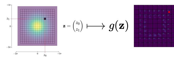
Figure 3: SnakeSynth generates spectral images from maps of quantile values sampled (in red) from two standard deviations of a Gaussian (normal) distribution in an arbitrary 2D coordinate grid. Grid interactions sample outputs from a restriction of the entire possible generator output distribution up to 95th percentile outcomes.
