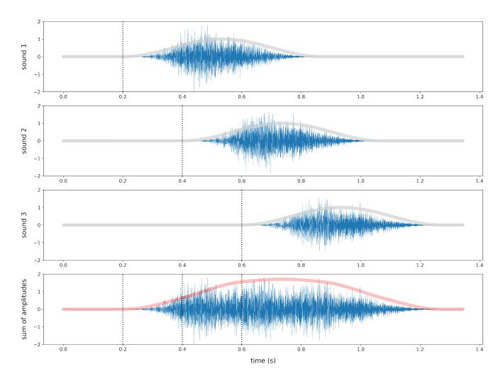
Figure 4: Time-triggered sound samples (first three rows) generated, windowed, and summed over time to produce a single variable-length sound (bottom row). Increasing amplitude by summing overlapping sound windows enables virtual mechanical "driving" through the SnakeSynth controller to produce resonance-like effects. The amplitude of the combined sound increases with greater sample overlap.
