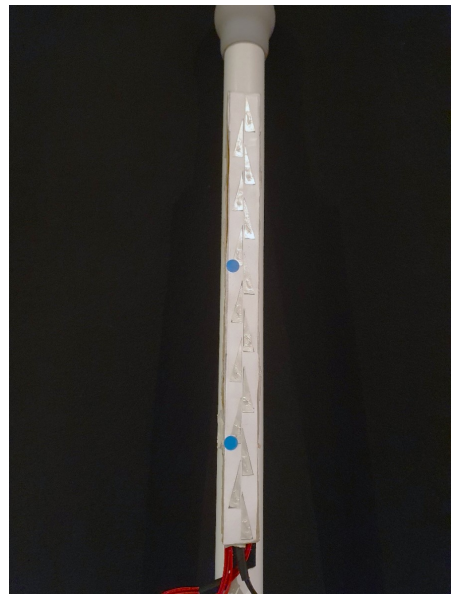
Figure 6: The capacitive sensor array mounted on the top of the handle.
