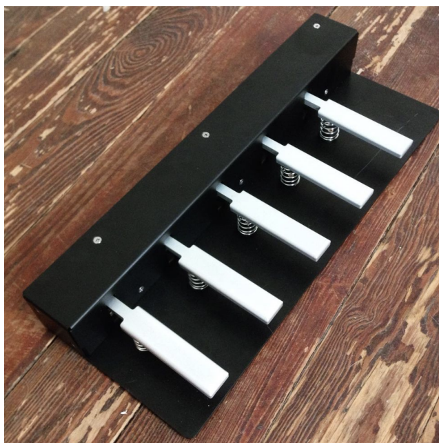
Figure 5: Photograph of the left-foot pedal system, with enclosure cover in place
