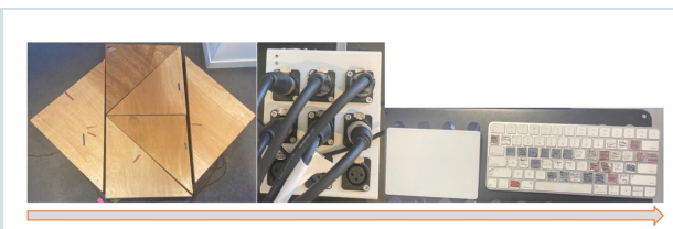
Figure 2. Floors and mouse/keyboard combination. Control voltages are sent from the Floors to a Teensy inside the controller box (middle), which sends MIDI CC and pitch bend to Max and Ableton. Layers of sound, channels, effects chains are mapped to MIDI CC, enabled via key
