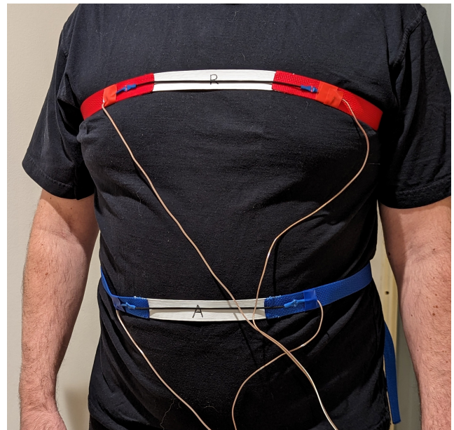
Figure 2: ATEM-P abdominal (blue) and ribcage (red) belts.
