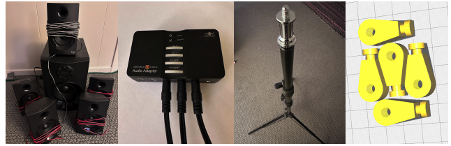
Figure 2: Left to right: combined sub and amplifier unit and 5 speakers, 7.1 channel audio interface, photography light stand, threaded mounting adapters.
