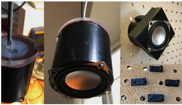
Figure 10: Left/center: A PVC speaker enclosure with dacron insulation, rubber gasket, and laser cut backing, meant to hang from above by string. Right: 3D-printed speaker enclosure designed to be mounted through pegboard holes, with peg and clip mechanism.
