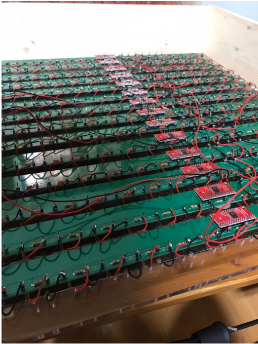
Figure 7: PCBs mounted on the inner part of the interface
