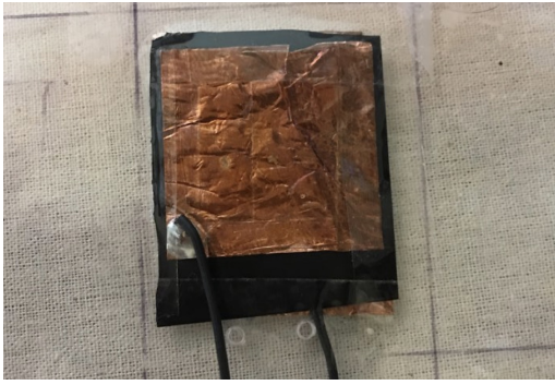
Figure 4: The upper layer copper tape and Velostat taped on the bottom layer copper tape.
