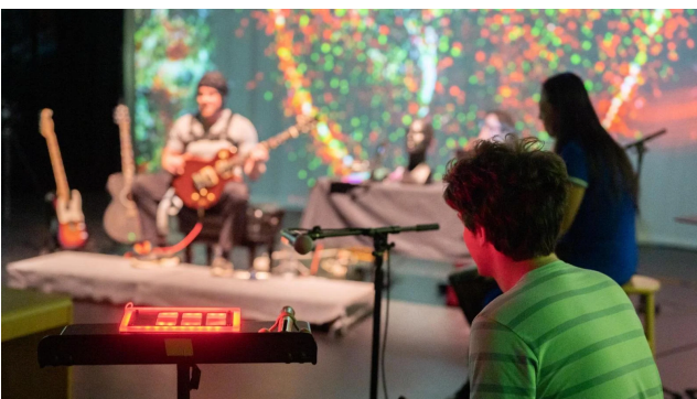
Figure 5: Color/ Chord selection controller (glowing red in image). Figure demonstrates a controller that already has a chosen color. The six buttons show 6 different colors when the controllers are ready to have a color selected. Rhythmic instruments of various kinds are located near the controller stations. Controllers are shown resting on top of music stands.
