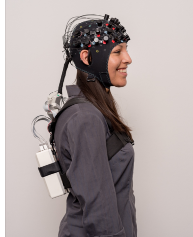
Figure 2: fNIRS device being worn. https://NIRx.net
