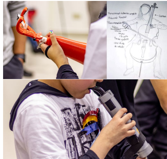
Figure 4: Upper panel: The resulting instrument for the "virtuoso follower" performer was a prosthetic forearm that would allow them to play the conventional cello. At the right side is shown the original design proposed by the design team. Lower panel: For the "energetic improviser" the design team developed a one-handed MIDI flute that was connected to a synthesizer software allowing the performer to explore a wide spectra of timbres.
