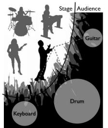
Figure 1. Conceptual model of SSN system. Spatial sound control is implemented through speakers of each audience's mobile phone. Performer decides the sound source location and influence
