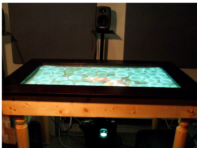
Figure 1: Our first-generation multi-touch table, using the Laser-Light Plane (LLP) method.
