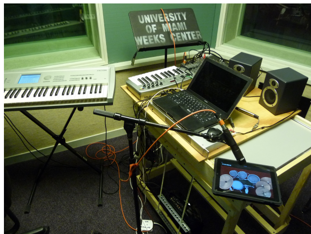
Figure 4: Experimental setup for testing latency times for our second-generation multi-touch table and other devices.
