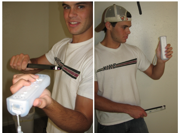
Figure 1: The orientation of the Wii remote determines whether the Wiiolin performs as a violin or cello.
