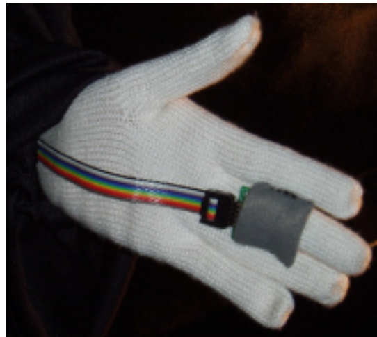
Figure 1: Accelerometer attached to hand
